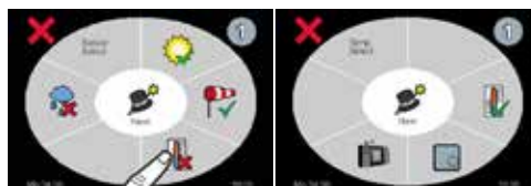
15. Selection of temperature sensors 16. Assignment of temperature sensors: internal temperature sensor display box, TE Indoor, TE Outdoor or TS Pro XL
